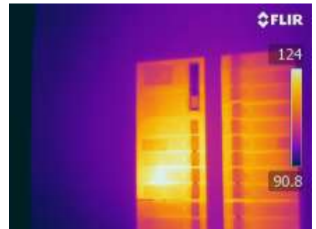
Heat images on house main panel breakers
