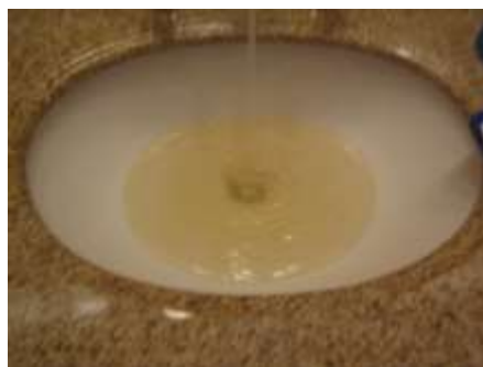
Rust from steel water piping
