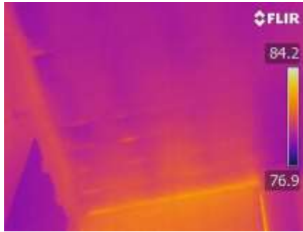
No anomalies on ceiling of family room with stains
