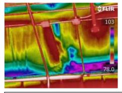
Images of water in insulation along west side warehouse
