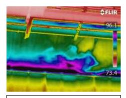
Water image in east warehouse on insulation under roof (same above)
