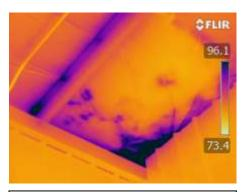
Water images on insulation at rear northeast corner
