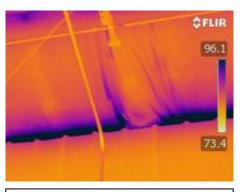
Image of bubble in insulation with suspect water
