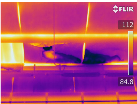
Images of moisture from active roof leakages on insulation
