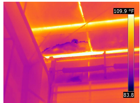
Images of moisture from active roof leakages on insulation
